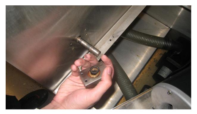
8. Remove the roller bar by pulling it back towards the motors until the other side is freed, then push the free side down at an angle and pull the other end of the roller through the hole.
