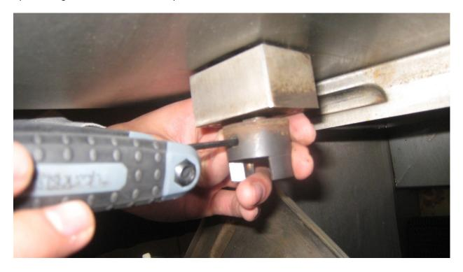
6. There are 4 screws holding the block to the wall of the chilling bay that need to be removed. There are 4 acorn nuts on the other side of the chilling bay wall holding the block in place that need to be secured to remove the screws.
