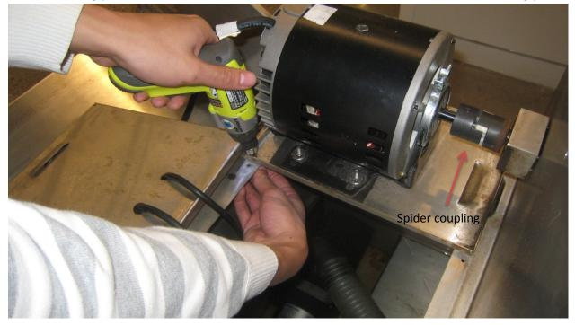
5. Back the motor mounting plates with the motors still attached enough so the spider coupling separates into two hubs. Remove the hub situated near the chilling bay wall. The hub can be removed by loosening a set screw with a hex key.
