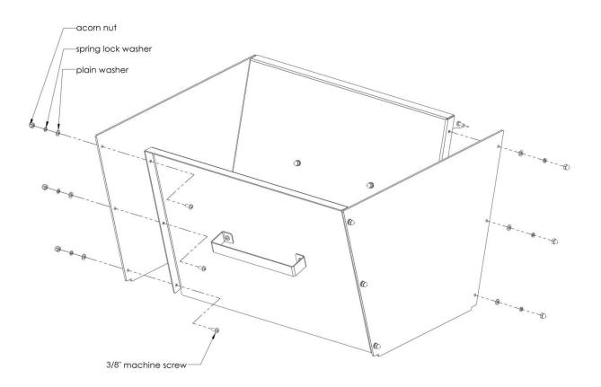
4. The completed ice chute should be similar to the one in the picture below. The nuts and bolts should be checked to be tight once a week.
