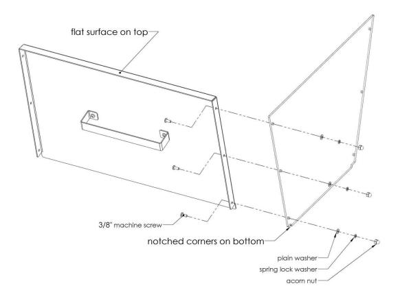
3. Attach the two halves of the ice bin together as shown in the figure 3/8" machine screws. Tighten each machine screw using a screwdriver while holding the acorn nuts in place with a wrench or pliers.
