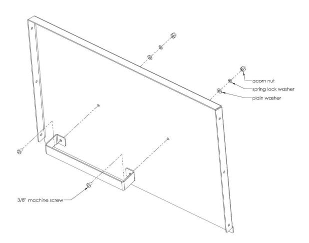
2. Attach one of the clear plastic sides to the metal plate using 3 of the 3/8" machine screws as shown in the figure below. Note the location of the notches in the plastic relative to the plate. Tighten each machine screw using a screwdriver while holding the acorn nuts in place with a wrench or pliers. Repeat the process for the other stainless steel plate and plastic sheet.
